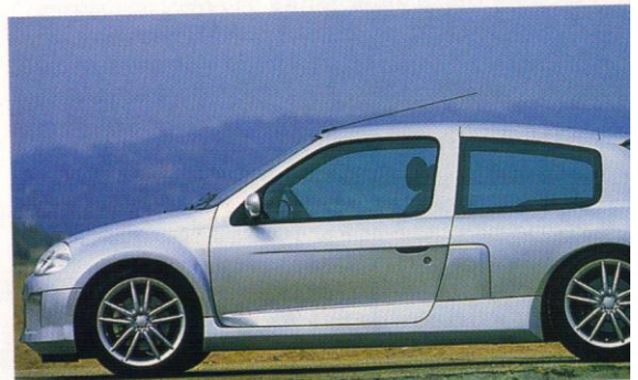
Same overall length as regular car, but tracks much wider
