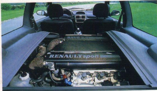
Mid-mounted 3.0 V6 is from Laguna, uprated to 250bhp
