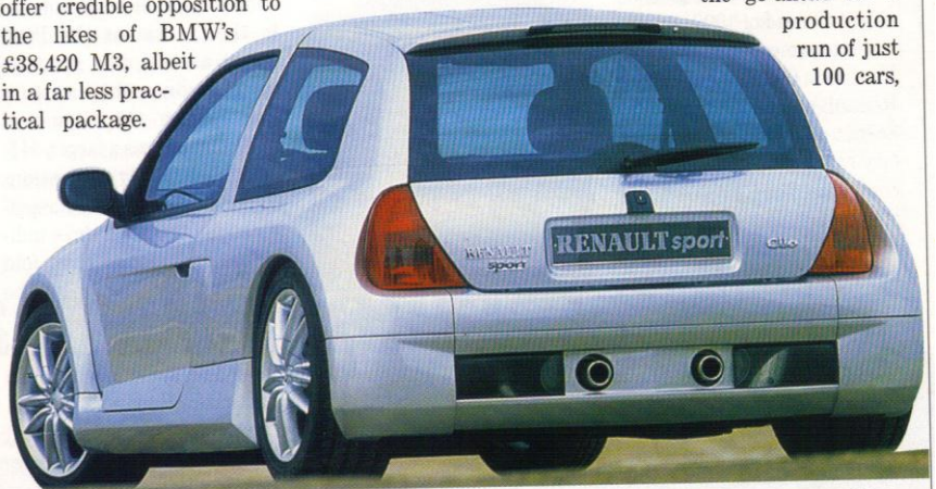
Rear hatch, bonnet and roof are from cooking Clio, but other body panels are composite
